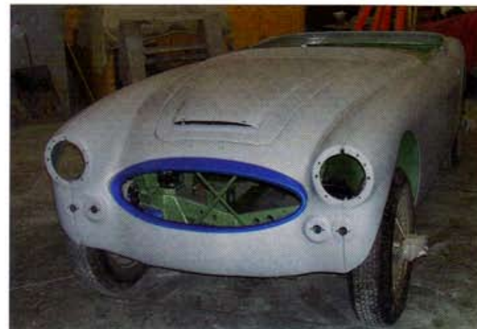
When Peter was satisfied with the fit of the panels, he sanded and degreased each panel and sprayed it with PPG DP40 epoxy primer. He then reassembled the body and trailered the car to the paint shop.
