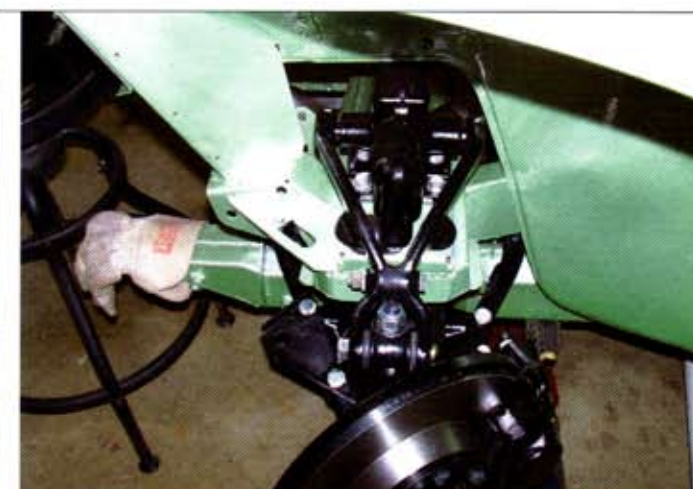
All of the suspension components were sandblasted, primed and finished in black Shop-Line two-part urethane. Original fasteners were cleaned and given new zinc plating, using a kit from Caswell.
