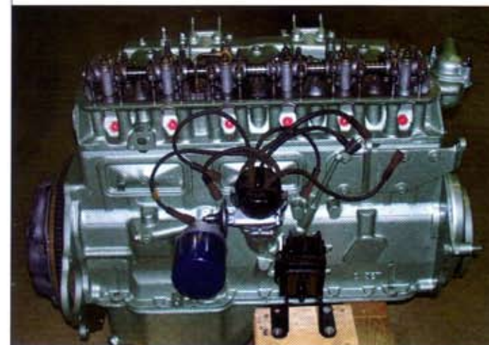
While Peter was doing the bodywork, Mike's Motor Services was rebuilding the straight-six, which needed a slight overbore. Peter finished the engine in the correct color, with paint from Moss Motors.
