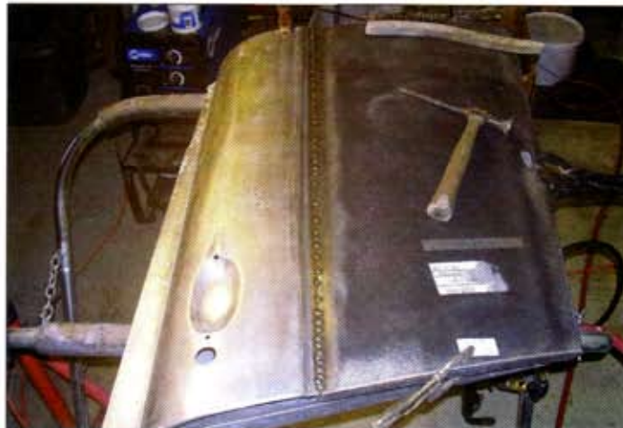
Lower door skins from Kilmartin Automotive Sheetmetal were welded into position, using a 110-volt Miller 125 MIG welder. A series of initial tack welds kept the panel from overheating and warping.
