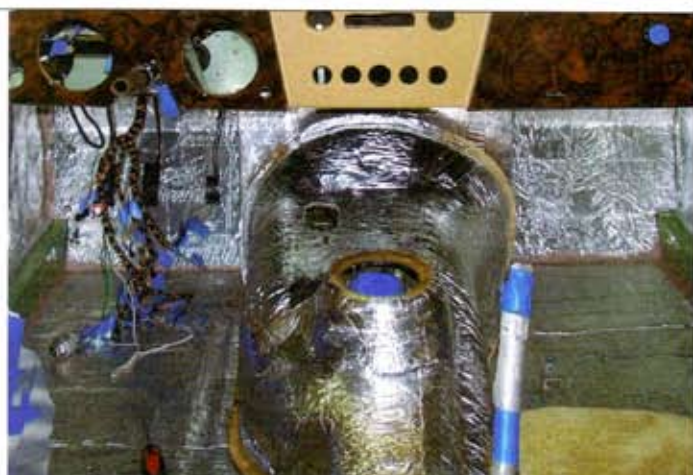
The floors, transmission tunnel and firewall were all covered with Dynatex to keep heat and noise out of the cabin. Healey Wood supplied a new dashboard; Peter reupholstered the center section in leather.
