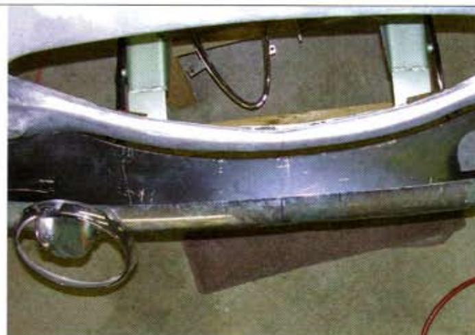
The aluminum front shroud had to be carefully shaped to create a perfectly even gap with the reproduction steel splash panel. The openings for the grille and headlamps required similar attention.
