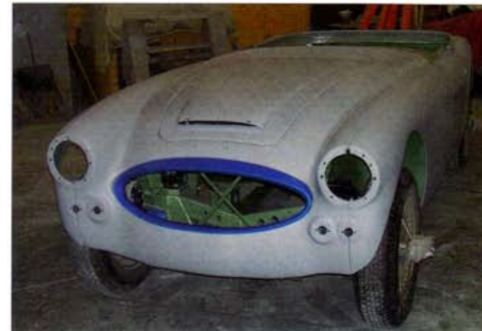
When Peter was satisfied with the fit of the panels, he sanded and degreased each panel and sprayed it with PPG DP40 epoxy primer. He then reassembled the body and trailered the car to the paint shop.
