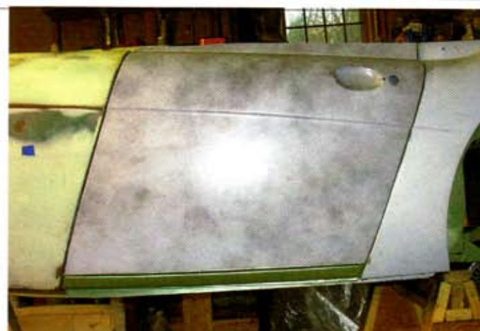
In addition to the door gaps, there were many, many elements between the door and the fenders that had to meet up perfectly. This was one of the most time-consuming, but vital, parts of the restoration.
