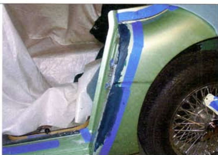
With the car nearly complete, Peter decided he could not live with the fit between the doors and back fenders. He ground off the new paint and reshaped the edge, then had the fenders painted again.
