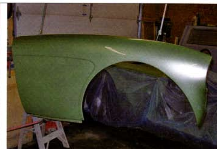
The body panels were sprayed with three coats of PPG Deltron 2000 basecoat and three coats of PPG 2021 clearcoat. The panels were oriented as they would be on the car.
