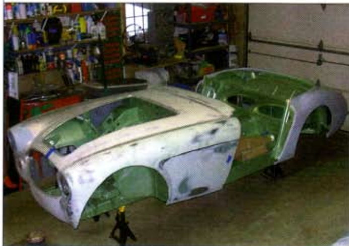
The bolt-on body panels were lightly assembled onto the frame/bulkhead unit countless times as Peter adjusted the fit. He began at the back of the car, and worked his way to the front.
