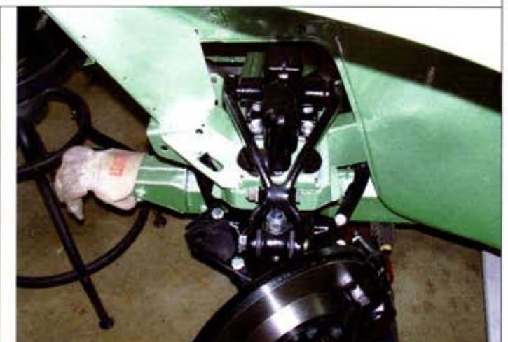
All of the suspension components were sandblasted, primed and finished in black Shop-Line two-part urethane. Original fasteners were cleaned and given new zinc plating, using a kit from Caswell.
