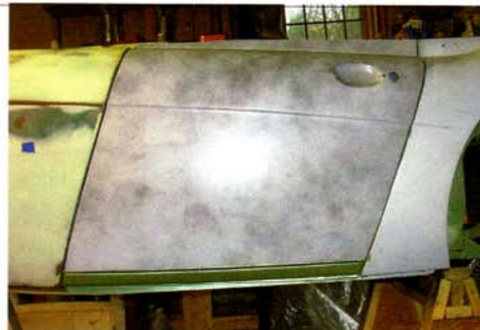
In addition to the door gaps, there were many, many elements between the door and the fenders that had to meet up perfectly. This was one of the most time-consuming, but vital, parts of the restoration.
