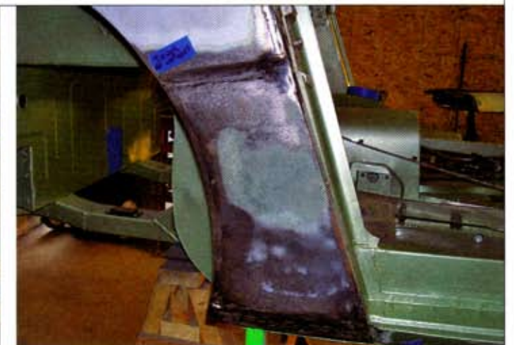
Peter cut away the corroded lower quarters of the rear fenders, and welded in patch panels he had fabricated. He rolled the lip of the panel around a piece of brazing rod, recreating the original look.
