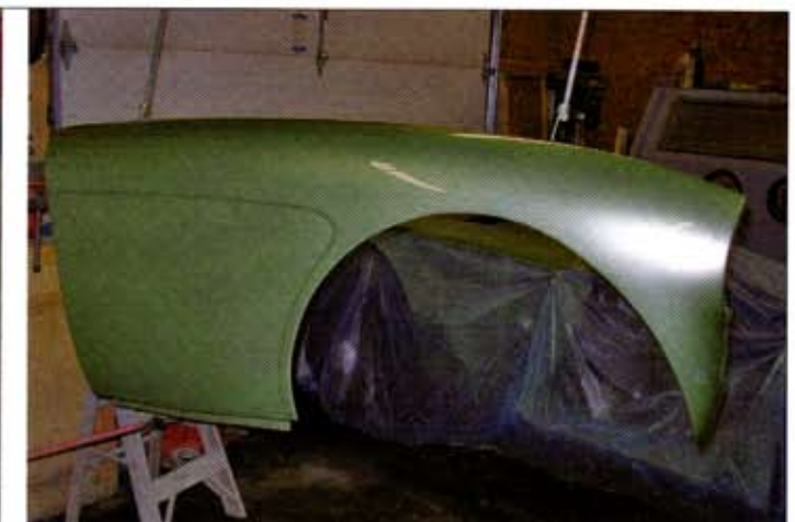
The body panels were sprayed with three coats of PPG Deltron 2000 basecoat and three coats of PPG 2021 clearcoat. The panels were oriented as they would be on the car.
