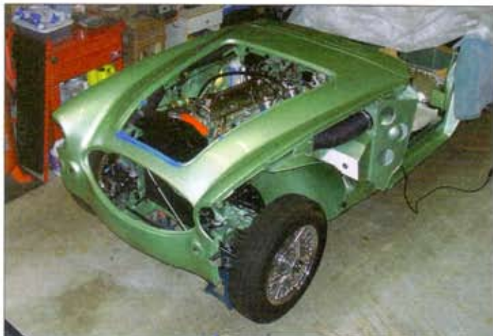
With the drivetrain and suspension in place, the freshly painted body panels could be bolted on. The front shroud had been safely hung from the roof of the garage until the time came for its installation.
