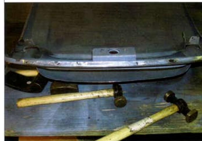
Hammer-and-dolly work was one of the skills Peter taught himself during the restoration. Here, the front edge of the hood is shaped, so that it will perfectly line up with the opening in the front shroud.
