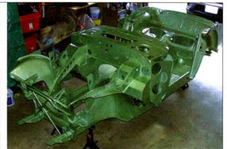
Jule Enterprises welded the car's original front and rear bulkheads to a stronger, reproduction frame, and applied the Opaline Metallic Green finish Peter had chosen. The work was done in seven weeks.
